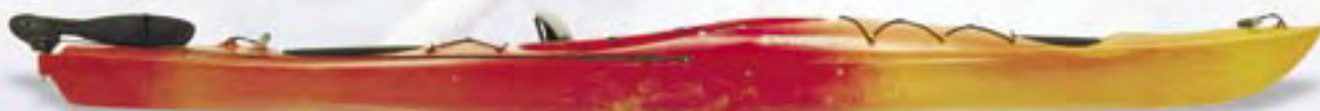
CATALYST 12.8 Length: 12'10" • Width: 25" Weight: 45 lbs. • Maximum Load: 275 lbs. Cockpit: 38x21" • Deck Height: 11" Storage Capacity (bow/stern): 2400/4150in 3
